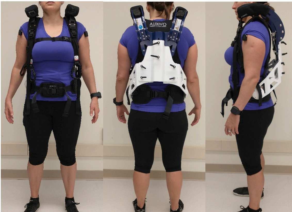
Fig. 1. A participant wearing the Auxivo CarrySuit (Auxivo AG, Switzerland): front, back and side views. The participant is also wearing the sensors used in the study: a heart rate wristband and electromyography sensors on the shoulders, lower and upper back (not visible).
