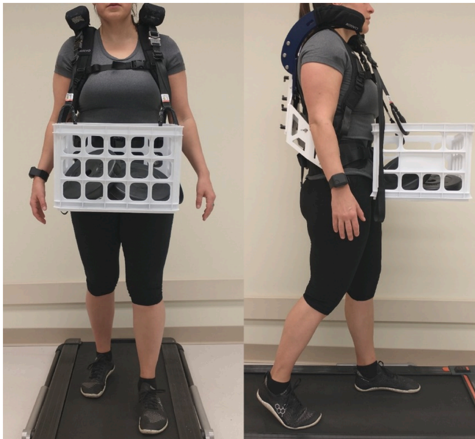
Fig. 2. A participant carrying the box with the exoskeleton on the treadmill, front and side views.
