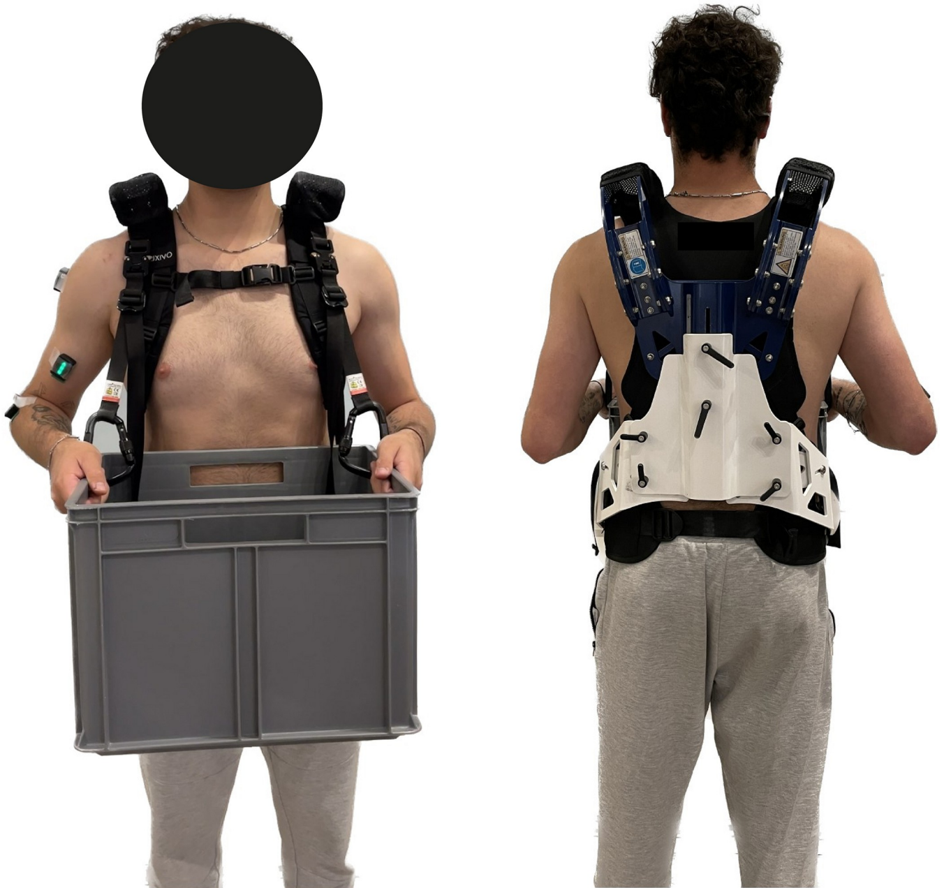
Fig 1. Participant wearing Auxivo CarrySuit and EMG sensors.
