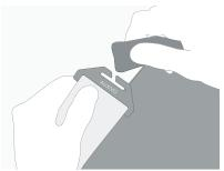
Start by inserting the longer side of the EES hook into the loop of the upper connecting strap.
