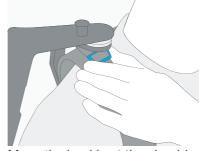
Move the buckle at the shoulder upwards to increase the stability of the attachment between shoulder structure and vest.
