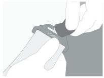
First, remove the back EES by pulling the textile band to one side of the metal hook.
