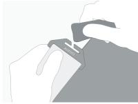
When the textile band slips out of the hook, pull it out. Repeat the process for the other connection.
