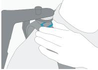
Move the buckle at the shoulder upwards to increase the stability of the attachment between shoulder structure and vest.
