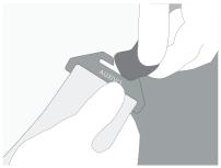
Then squeeze the loop onto the shorter side of the hook. Repeat the process for the lower connection and the other side.
