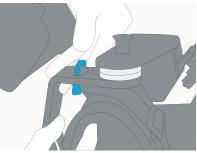
Attach each shoulder attachment buckle to the slot on each back structure.
