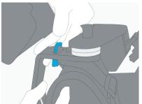
Tilt and push the attachement buckle through the slot in the back structure.
