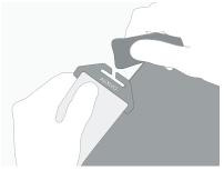
Separate all the textiles, rigid parts and back elastics prior to washing.
