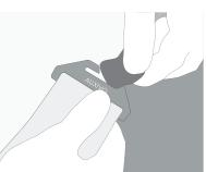
When the textile band slips out of the hook, pull it out. Repeat the process for the other connection.
