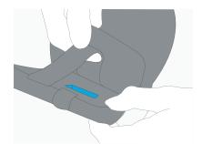
Detach the Velcro strap on the bottom of the arm cuff, and pull the textile cover off the arm cuff.
