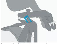
Insert the back structures into their vest pocket. Attach each shoulder attachment buckle to the slot on each back structure.
