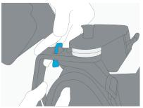
Separate the textiles and rigid parts prior to washing. First, tilt and push the buckle through the slot in the back structure.
