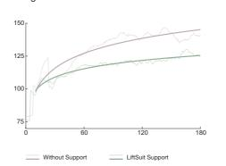
The average heart rate while repetitively lifting loads without the exoskeleton was 122 bpm. This was reduced to 117 bpm when working with the LiftSuit. The associated cardiac cost was reduced from 58 to 54 bpm, implying a 7% relief for the cardiovascular system.
