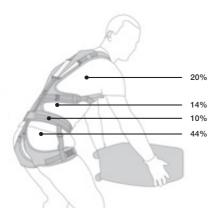
Averaged across all participants, the rate at which the median frequency sinks was significantly lower when wearing the LiftSuit. In the study, the support of the LiftSuit reduced the rate of fatigue by 44% in the hip muscles and by 10% in the lower back while holding a heavy box in a forward-leaning body position.
