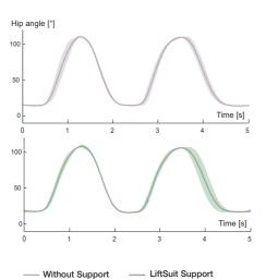
The minimum and maximum hip and knee angles remained unchanged during lifting movements when using the LiftSuit. These results suggest that the participants did not alter their motion patterns and performed ergonomic lifting movements.
