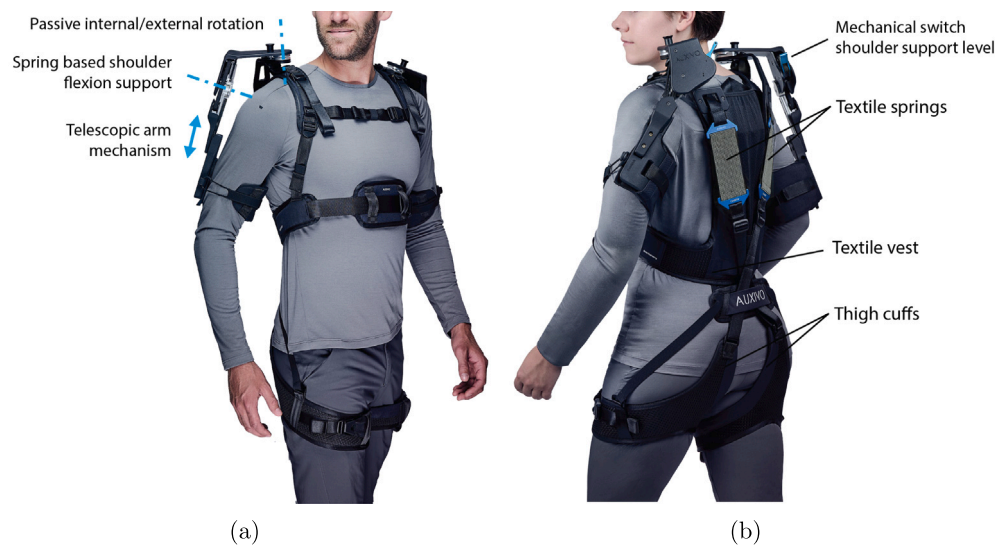
Fig. 1. The OmniSuit back and shoulder support exoskeleton from the front (a) and back (b).
