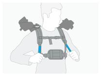
Tighten the shoulder straps to make sure the vest is worn high on the torso.
