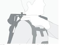
When gap between shoulder and exoskeleton is less than two fingers, tighten shoulder straps more (step 3).
