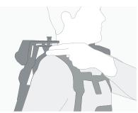
When gap between shoulder and exoskeleton is less than two fingers, tighten shoulderstraps more (Step 4).
