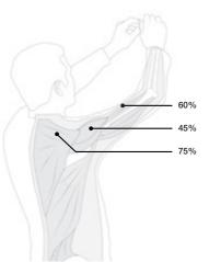
The back support module reduced the rate of fatigue by 44% in the hip muscles and by 14% in the lower back while holding a heavy box in a forward-leaning body position.
