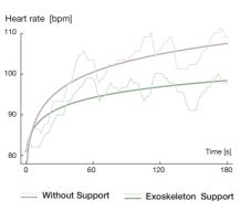
Cardiac cost of fastening screws with a powered drill above the head was 21 bpm. During the study using the shoulder support module reduced the cardiac cost by 15% to 18 bpm.
