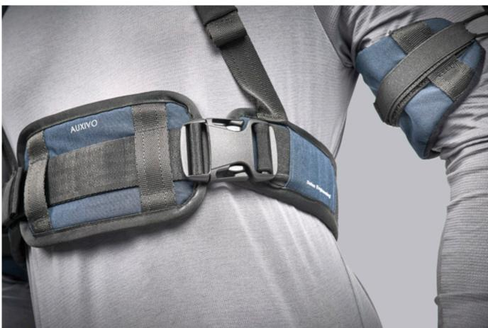
The split-vest design ensures high freedom of movement and serves as an interface between the wearer and the mechanical structure. Choosing the thorax, rather than the hips, as the attachment point between the human user and the exoskeleton allows unconstrained spine movement.
