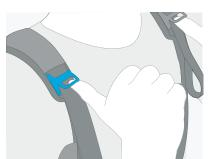
To deactivate the support lift the deactivation buckles and simultaneously lift the left and then right leg.
