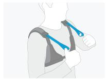
To activate the back support pull on the looped activation straps.
