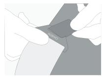
Remove the back EES by pulling the textile band to one side of the metal hook.
