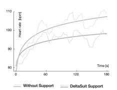
Cardiac cost of fastening screws with a powered drill above the head was 21 bpm. During the study the support of the DeltaSuit reduced the cardiac cost by 15% to 18 bpm.
