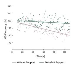
Over all participants the rate in which the median frequency sinks was significantly lower when wearing the DeltaSuit. In the study the support of the DeltaSuit reduced fatigue by 45% in the shoulder muscles, 60% in the upper arm and 75% in the neck while holding a power tool above the head.
